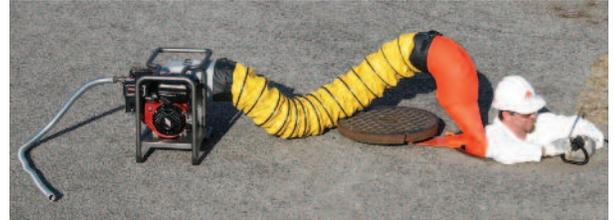
**Application:** In order to stabilize the atmosphere in the confined space, continuous ventilation should be used before and during occupancy of the confined space. These blowers can be used to provide fresh air to underground vaults, tanks, open pits, and many other similar areas.
