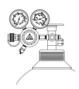
Note: Reserve air must be at least Grade-D breathing air, and must be set at a minimum of 50psi, but not to exceed 125psi.
