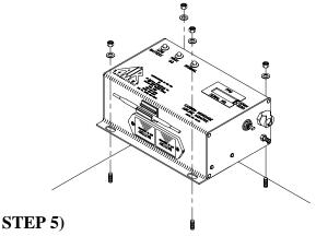
Reassemble monitor and install back into system. Connect all external connections. Allow monitor to stabilize and recalibrate.
