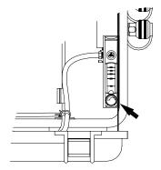
When the CO concentration level exceeds the alarm set point, the green "NORMAL" light will turn off, the red "HIGH CO" light illuminates, the audible alarm will sound, and the remote alarm connections will energize.
