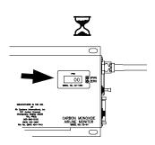
5. Adjust the "span" pot adjustment screw (clockwise to increase, counterclockwise to decrease) until the digital display reads the same concentration (ppm) as printed on the calibration gas cylinder.
