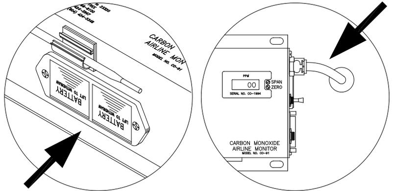
**Note:** The 9 volt batteries continuously provide a required bias voltage to the CO sensor and power the monitor. If power is removed for a period of 2 hours or more, a 1 hour restabilization period is required for the sensor as erratic readings may occur.
