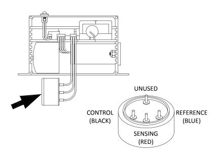
Step 4) Remove sensor from sensor cup and remove leads. Take the new sensor and remove the metal spring. Reattach leads to the proper colored terminals on the new sensor. Install new sensor into sensor cup.
