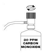
THE MONITOR IS NOW CALIBRATED AND SHOULD BE RECALIBRATED MONTHLY OR IF ACCURACY IS QUESTIONABLE. CHECK LOCAL REQUIREMENTS AND RECALIBRATE AS REQUIRED.
