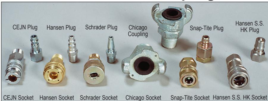
Almost all manufacturers make an industrial interchange style. A 1/4" industrial interchange from Hansen will be compatible with a 1/4" industrial interchange from either Parker or Foster. If a customer states they are in need of a Foster fitting, ask if it is a Foster Schrader or Foster Hansen style. We can cross reference additional fitting types; please provide part numbers imprinted on the socket or plug.
