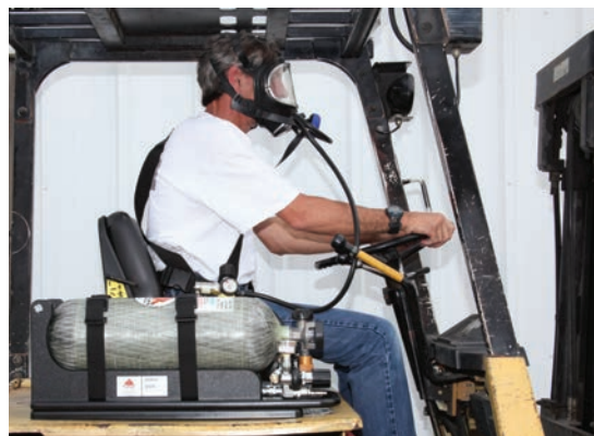
PAK-SFL™ mounted on forklift
