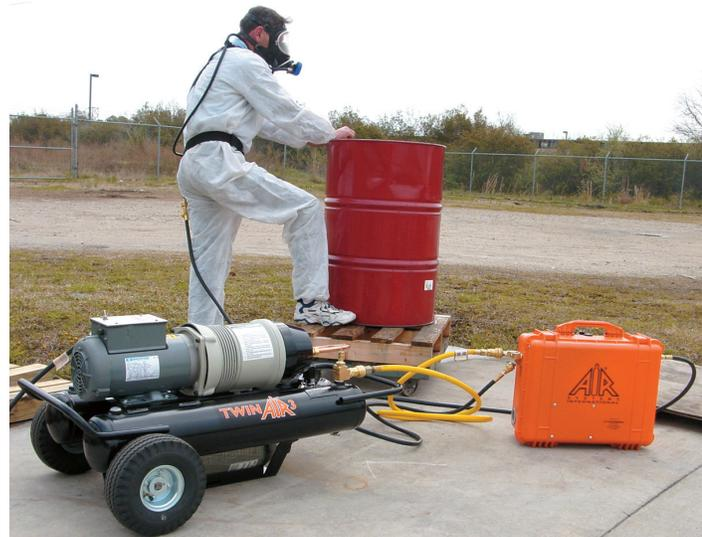
**NIOSH requires the use of a 5 minute airline escape respirator when working in IDLH environments.**
