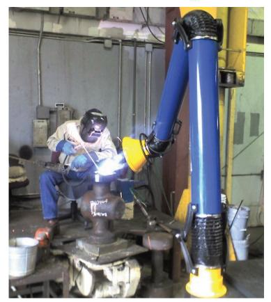
The Fume-Air<sup>™</sup> 750 HEPA filtered fume extractor provides a minimum flow of 750 cfm through the 13" hood making it ideal for welding and soldering applications where large flow volume is required.
