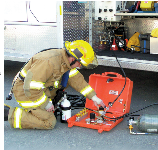
The MACK-2™ is ideal for emergency refilling SCBA cylinders from aerial command stations.
