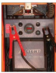
Direct connection from vehicle's battery system via jumper cables to battery posts located on the standard battery pack
